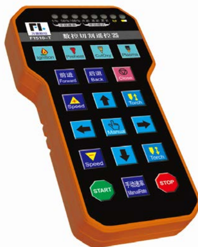
Fig.14.1 layout of remote controller
